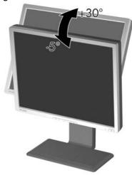
NOTE: The 24" model has a tilt range of -5 to +25 degrees.
