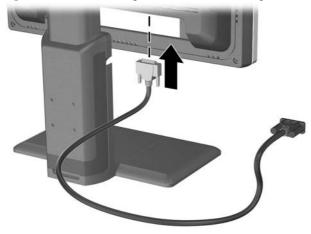
Figure 3-4 Connecting the DVI-D Signal Cable
