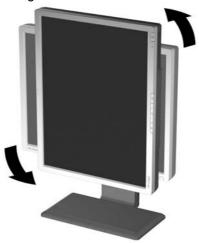
NOTE: The 20" model (shown above) pivots counter-clockwise; the 19" and 24" models pivot clockwise.
