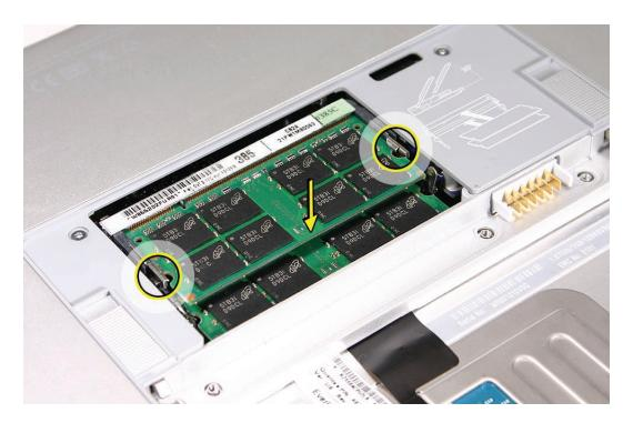
4. To ensure that the memory cards are fully and securely seated, for the lower card, use a black stick leveraged against the frame to evenly push along the back of the card.
