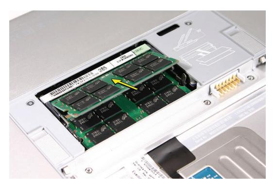
3. When the card is fully seated, push the card straight down until the tabs click onto both sides of the card, locking it into place.
