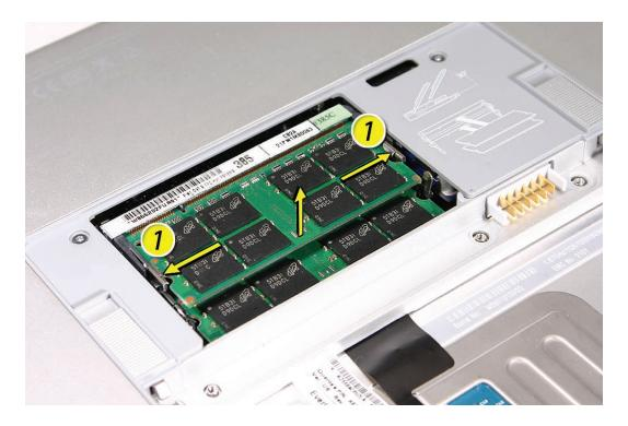
5. Pull the card straight back and out of the memory slot.
