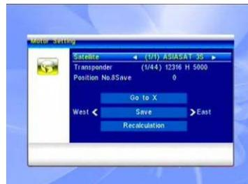
**Position No., & Save:** The range is from 0 to 63. "0" delegates the original position. You can select the proper value when you has rotated the antenna.
